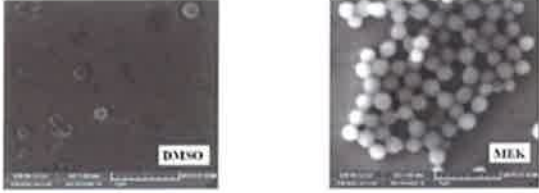
FESEM images of ultrathin multilayers of PVDF obtained using good (DMSO) and swelling (MEK) solvents at A-S interface.
