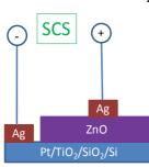
We have taken up the systematic study of resistive switching of Metal/ZnO/Pt devices with Ag or Al top electrodes.
