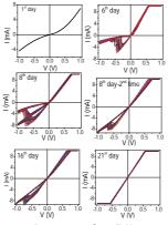
Resistive switching (I-V characteristics) study of Ag/ZnO/Pt device from 1st day to 21st day. Exchange bias and magnetoresistance of magnetic nanoparticles, such as, NiO, doped NiO
