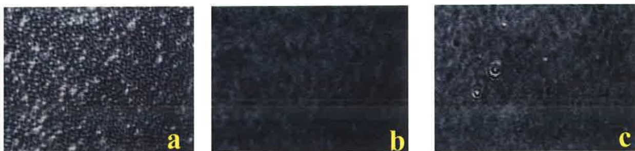
Figure 2: Brewster angle microscope images of Ni-PC phthalocyanine monolayer at the air-water interface. a) Gas + L_1 phase at 120.5 \text{ Å}^2 , b) L_1 + S phase at 69.2 \text{ Å}^2 and c) S + bulk crystallites at 50.2 \text{ Å}^2 at 25^\circ\text{C} . Field of view: 157 \times 157 \mu\text{m}^2 .
