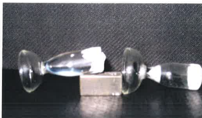
Left: Pure E7 Right: X=0.6 gel. Note the immobility of the gel due its high viscosity as against the freely flowing pure E7.
